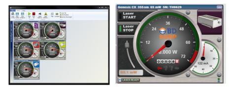
3. Click on Laser Start, verify laser is at 60mW (10-20 seconds). <u>You may need to click on Laser</u> <u>STOP first followed by Laser START for the laser to come on.</u>
